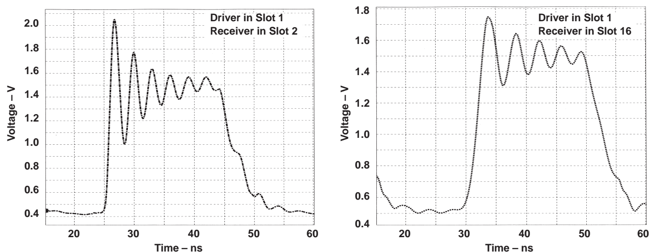
Figure 10. GTL16622A Signal Integrity (HSPICE Simulation Results)
